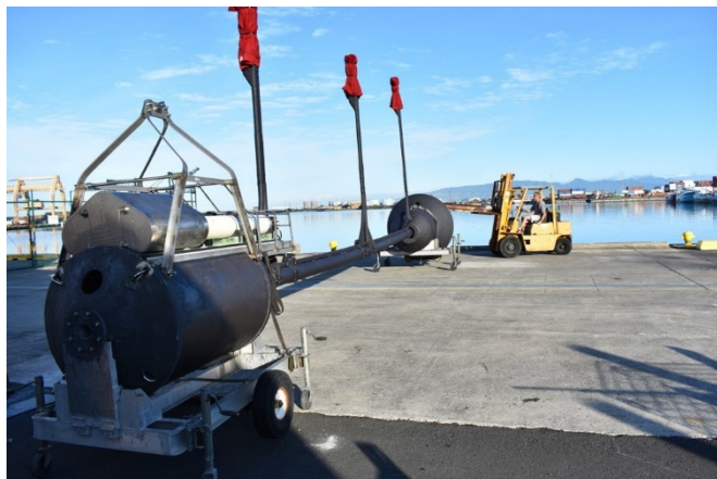
Figure 1: MOBY pre-launch, being brought out to the ship in the Univ. of Hawaii Marine Facility. The new dual spectrometer (the bright silver housing, along with the white spectrometer tubes) is attached on top of the MOBY instrument housing. It is about to be loaded onto the side of the R/V Ka'imikai-O-Kanaloa to be brought out to the mooring site near the island of Lanai, Hawaii.
